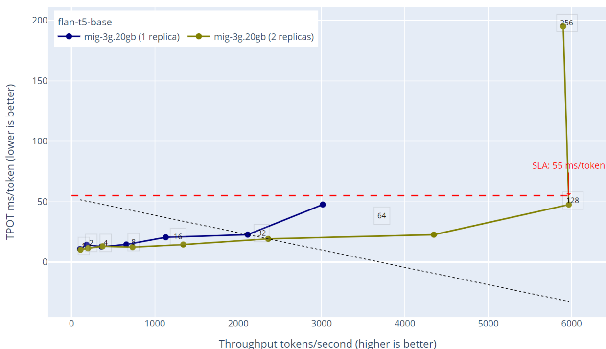
Figure 5. Performance comparison between deploying the same model in a single replica vs the maximum available replicas '3g.20gb' - flan-t5-base throughput over time-per-output-token
